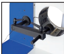
Back Limit Switch
